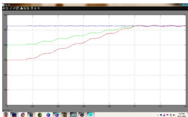
Fig.16 (b) dc-link voltage, for different initial values of the dc-link voltage, during downstream phase-A-to-ground fault.
