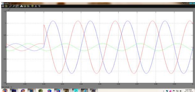
Fig.6 (b) Fault currents, during downstream phase-to-phase fault when the DVR is inactive (bypassed).
