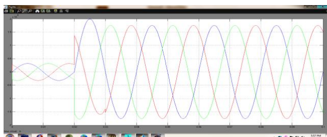
Fig. 4(b) Fault currents, during downstream three-phase fault when the DVR is inactive (bypassed).
