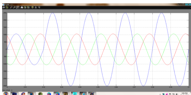
Fig.8 (b) Fault currents, during the downstream single-phase to-ground fault when the DVR is inactive (bypassed).
